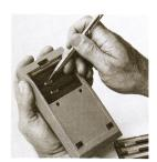
4. See if the battery connector springs on the calculator have been inadvertently flattened inward. If so, bend them out and try the battery again.
