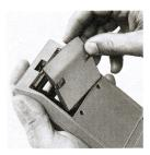
6. Insert the bottom of the battery door behind the retaining groove and close the door
