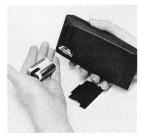
Place the new battery pack into the calculator. Your calculator will turn on only if the battery pack is inserted correctly.
