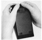
6. Turn calculator over and turn power on to assure proper battery installation. If the display does not light make sure the battery pack is correctly placed in calculator.
